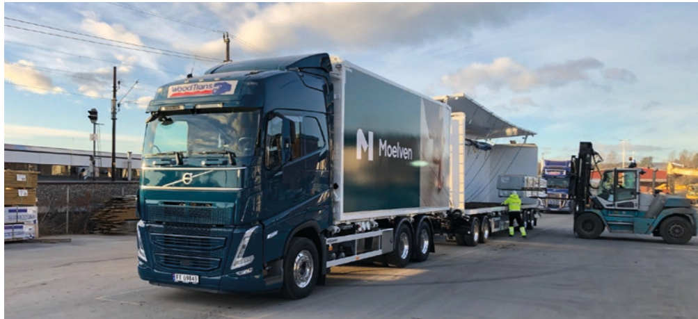
New trucks with modern engines that provide low emissions combined with high load capacity are important to reduce the climate footprint from distribution. The picture shows a modular vehicle combination that the company Woodtrans AS uses for the transport of chips and finished goods for Moelven.
