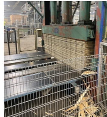
On 24 February 2023, the newly developed lignin-based adhesive for plywood production was tested at Moelven Vänerply AB. Both handling, application and pressing in the hot press went well. With this type of innovation project, Moelven is at the forefront in the development of plywood production. The new adhesive is fossil-free and therefore has the potential to significantly reduce the CO2 footprint and thus help make plywood an even more sustainable and environmentally friendly product. Photo: Stora Enso.
