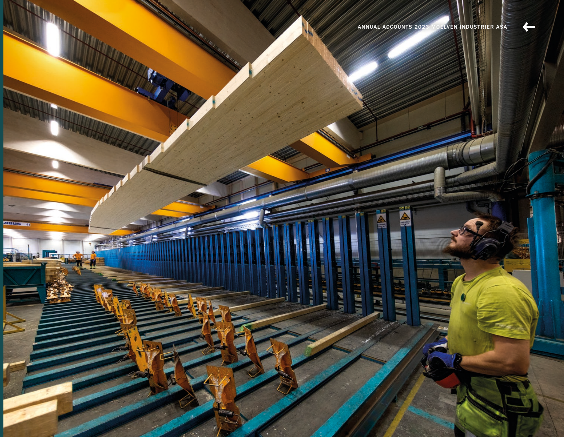
Elgiganten's new warehouse and logistics facility in Jönköping will be one of the largest in the Nordic region. Moelven's delivery consists of over 500 gable roof beams, and they are 24 meters long and almost two meters tall. The load bearing structure of the 86,000 square meter building consists entirely of glulam from Moelven Töreboda AB and Moelven Limtre AS. Photo: Sören Håkanlind and Jonas Ingman
