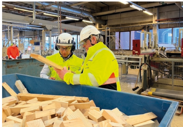
CEO Morten Kristiansen and system engineer Ahmed Nasrullah study pieces of raw material that have been mechanically identified and removed at Moelven Profil AS. The sorting is due to faults such as twigs, cracks, resin pockets, etc. Parts with approved quality are finger jointed and become wooden components for window production, while the removed pieces end up as raw material for bioenergy.
